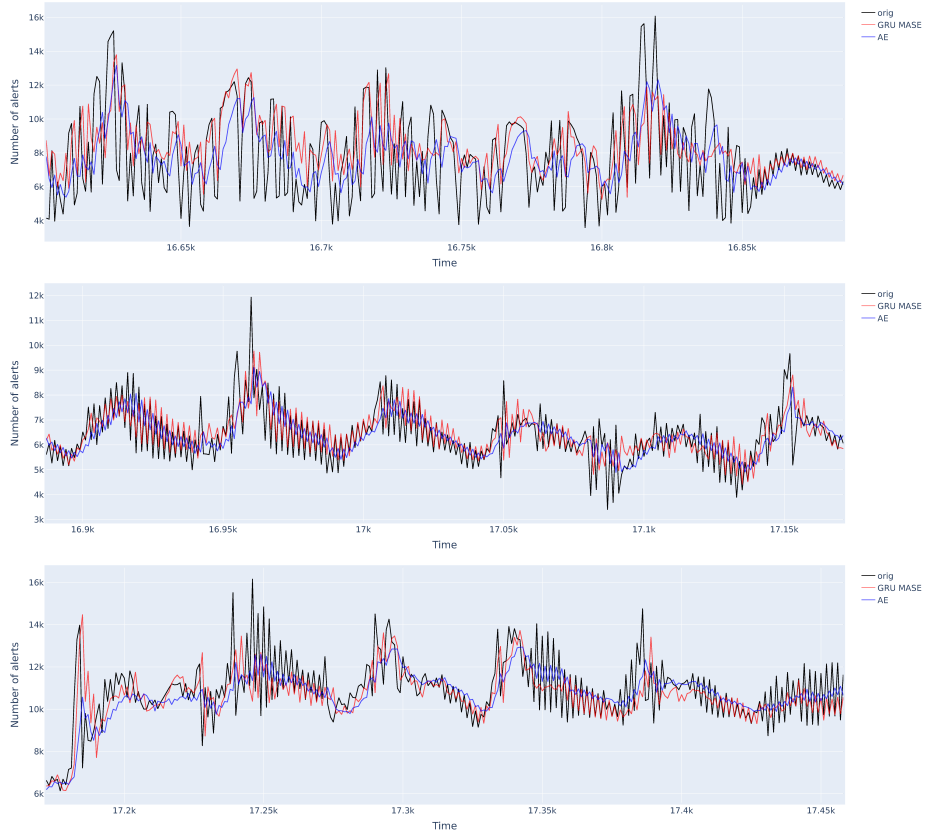
Fig. 2. Graphical comparison of best models based on neural networks (Gru with MASE loss) and statistical models (combination of ARIMA and Exponential smoothing) for port 445/TCP.
