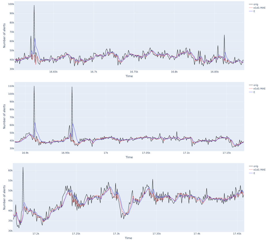
Fig. 1. Graphical comparison of best models based on neural networks (e1d1 with MAE loss) and statistical models (Exponential smoothing) for the total number of alerts.
